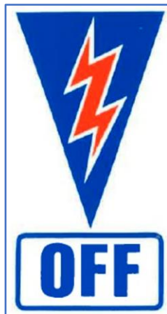
Figure 1: Required marking for kill switches
